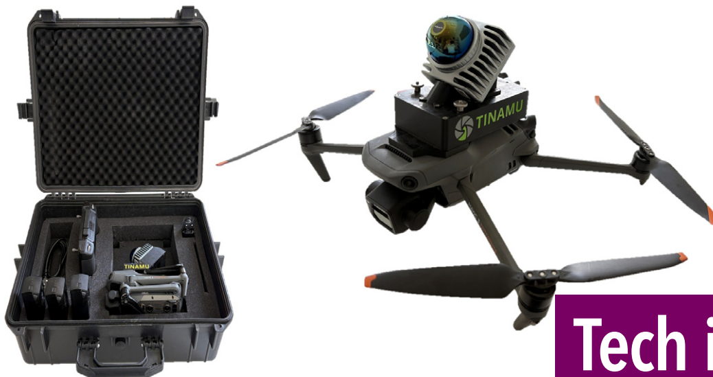
Left: The complete RMS Light system housed in a portable box. Right: A DJI Mavic 3 Enterprise equipped with the TINAMU sensor. The system is manually operated, and the generated point clouds can be uploaded directly for analysis and digital twin generation.
